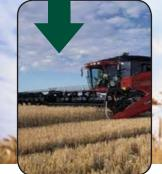
A combine is used to cut the wheat stalk. It also does the threshing, separating the kernels from the rest of the plant. The threshed grain is stored in a bin on the machine. The bin is emptied into a grain truck and taken to the grain elevator.
